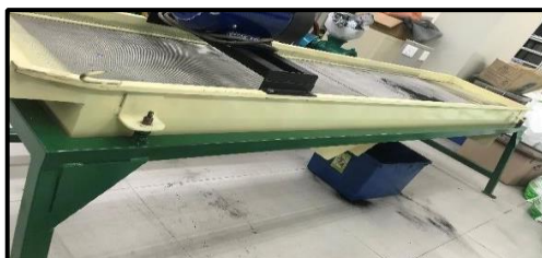
Figure 4. Sieving process of particle carbon
