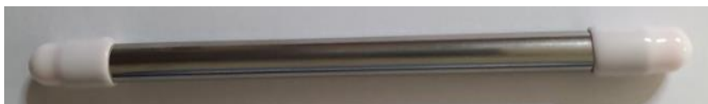
Figure 7. The sorbent tube physical appearance with palm shell activated carbon
