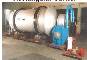
Pilot rotary burner
