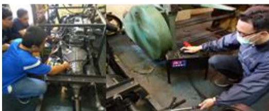
Figure 1. Opacity testing on diesel engine
